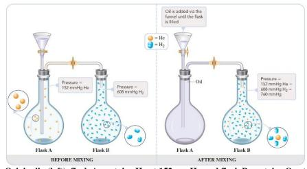
Originally (left), flask A contains He at 152 mmHg and flask B contains  $O_2$  at 608 mmHg. Flask A is then filled with oil forcing the He into flask B (right). The new pressure in flask B is 760 mmHg.
